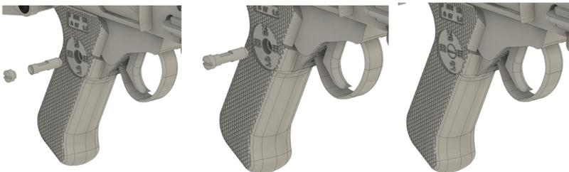
Glue Grip Pin Part 1 to Grip Pin Part 2, then carefully Push through the Hole in the Side of the Grip Handle past the Grip Spring. (DO NOT GLUE).
