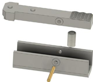
Place the 0.4 x 4 x 10mm Spring into End Cap Lock Part 1, then place End Cap Lock Part 2 into Part 1 and Secure with the 12mm x 1.5mm Brass Rod
