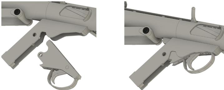
Carefully Slide the Trigger Housing up inside the Grip Frame. (DO NOT GLUE).
