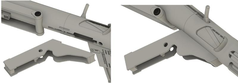
Glue the Grip Frame to the Underside of the Barrel.
