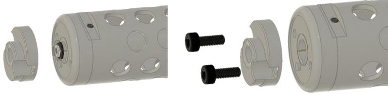
Fit the Fire LED into the Barrel Muzzle and Secure with Hot Glue. Next Secure the Barrel Muzzle to the Barrel Front End using 2 x M6 x 20mm Socket Head Screws
