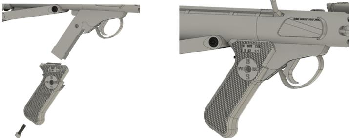
Slide the Grip Handle Over the Grip Frame and Secure in Place with either the 3D Printed M6 Bolt or a Real One. (DO NOT OVER TIGHTEN)
